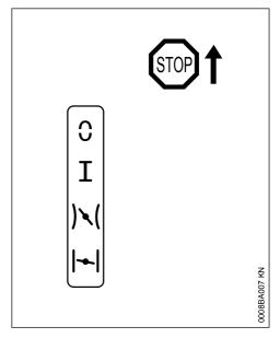
STOP or  ${\mathfrak O}$  – Master Control lever must be pushed in direction of STOP or  ${\mathfrak O}$  to switch off the ignition. When released, the Master Control lever springs back to the normal run position  ${\mathbf I}$  and the ignition is switched on again.
