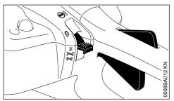
Press down the throttle trigger lockout and open the throttle – the Master Control lever moves to the run position I. After a cold start, warm up the engine by opening the throttle several times.
